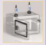
monitoring of relative humidity. Unit shipped with fittings, stopcock (for ¼" ID tubing) and instructions for easy assembly by user. Door opening: 23.6W X 12.7cm H (9.3W X 5"H). Overall dimensions: 33.8W X 25.4D X 21.6cm H (13.3W X 10D X 8.5"H). Internal volume: 0.35 cu. ft. Shipping weight: 3.0 Kg (6.6 lb.)
